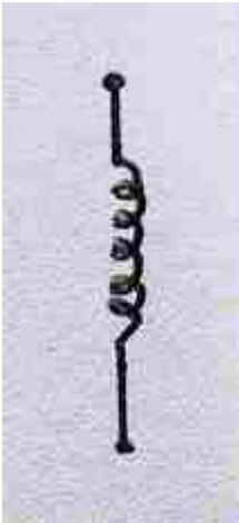
**BOBINA (INDUTOR) COM NÚCLEO DE AR**
